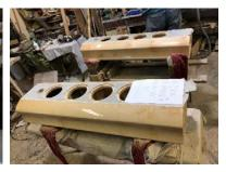
A view into Ayon's cabinet trademark: The "not damped" elliptical Ayon instrument plywood cabinet with its unequalled all-around radiating characteristics – by means of the elongated elliptical front plate the sound being carried into the room far and quasi "all around". In the new Ayon Speaker Series we also wanted to use organic and natural material to the greatest extent possible.
